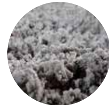
Struvite crystals from PHOSPAQ™
