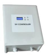
Single Lamps management Lamps' fault and elapsed life alarm via led and relay Increasing total hours meter for plant life Partial resettable decreasing hours meter for lamp life Stand-By command via "OK" button Flow meter ON/OFF command Change lamp counter (increasing) White/Blue 2×8 characters backlight display Potential free alarm relay 1A @ 30Vdc; 0,250A @ 230Vac Audible beeper for alarm (optional)
