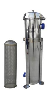
Housing for bag filters in AISI 304 (optional AISI 316), suitable for Size 2 length bag and equipped with a basket for the bag insertion.
