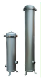
Housing for cartridge filters in AISI 304 (optional 316), in 2 different models with V-Band clamp or a middle closure system. They can accept DOE or 222 fin/flat cartridge of 20" 30" 40" length and come with poly coat finishing and are provided with 1/4" vent/drain port.
