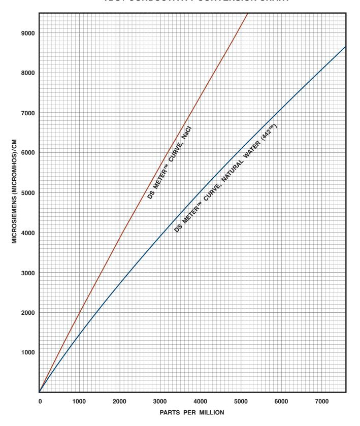
**Note:** The 442<sup>™</sup> to Conductivity correlation is non-linear and no single multiplier can be used to determine the relationship.
