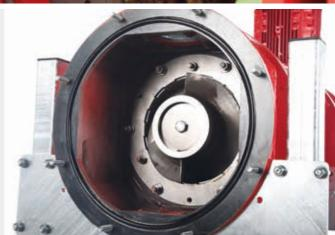
The easily accessible maintenance port provides very easy access to the press screw and sieve basket at any time.
