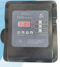
The electronic circuit allows the connection of an electrovalves to the waste (NC), a safety protecting the pool and avoiding water discharge during backwash. The electronic circuit allows also a connection to a pump which can either be set to stop during valve position change or to keep running.
