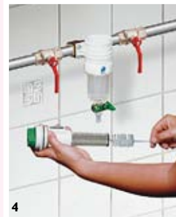
4. Brush the cartridge under the water using the special swab provided: if necessary, put the cartridge into 100 °C water or replace it. 5. For re-assembling, insert the diverter+cartridge assembling, insert the ring nut and rotate it clockwise until it is tight. 6. Turn on the water at the both side of the filter.
