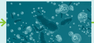
6. Bio Reaction Zone ensures that invading microorganisms are stopped and destroyed by disinfecting agents formed in the BacTerminator® disinfection chamber.
