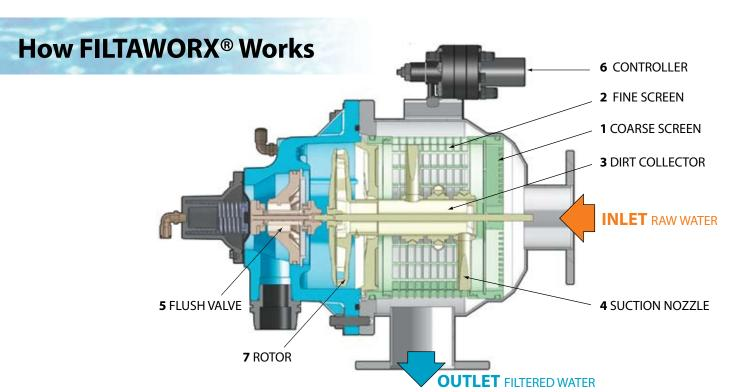
During normal filtering mode the raw water enters the Inlet of the filter, passes through the Coarse Screen (1), (this removes large debris that may obstruct the lower mechanism). Water then travels to the inside and through the Fine Screen (2) to the Outlet.
