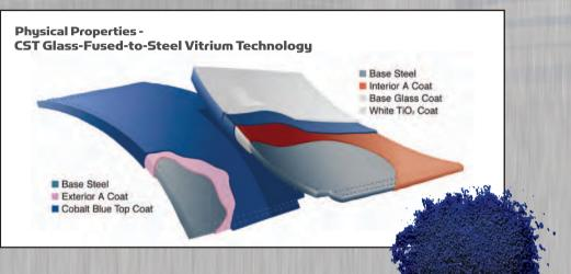
hard, inert barrier on both the interior and exterior tank surfaces guards against corrosion. Impermeable to liquids and vapors, it controls undercutting caused by corrosion and offers excellent impact and abrasion resistance.
