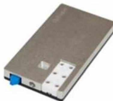
Figure 1. The MiniLab cartridge contains the optical chip and the microfluidic flow cell and is docked into the MiniLab system. The outer dimensions of the cartridge are 60x110x12 mm.
