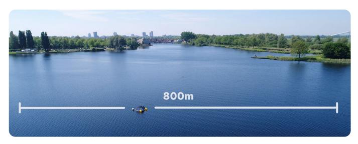
Each MPC-Buoy device can control algae in areas up to 800m in diameter.
