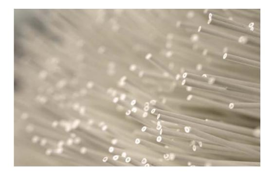
As a result of Hyflux's continuous efforts in research and development, the new Kristal<sup>®</sup> ultrafiltration membranes that now makes use of the reinforced PES fibres have achieved higher levels of tensile strength and better membrane performance.
