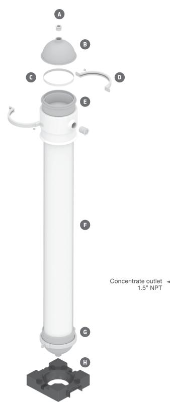
Each Kristal<sup>®</sup> module is a collection of thousands of Kristal<sup>®</sup> UF hollow fibres secured on both ends by a proprietary composite potting material and enclosed in a compact PVC housing.
