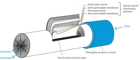
The flat sheet membranes are being rolled up around a permeate tube in order to form a spiral wound element. In membrane systems the elements are placed in series inside of a pressure vessel. The concentrate of the first element becomes the feed to the second element and so on.
