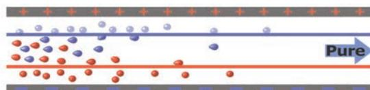
**Regeneration:** Feed water flushes through the cell at a lower flow rate, while electrode polarity is reversed. Ions are rejected from the electrode surface, concentrated in the flow channel, and flushed from the cell.
