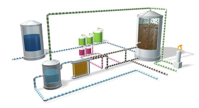
After anaerobic treatment, the UF membrane unit separates the clean permeate from the biomass.
