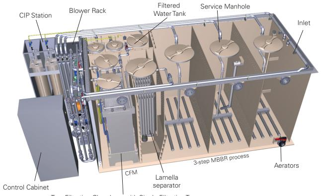
Two Filtration Chambers with Single Filtration Towers
