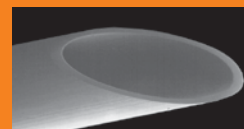
Microporous hydrophobic hollow fiber membrane
