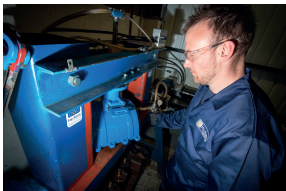
Automated Pneumatic Pressure Test Rig for Hi-Flow Performance Testing
