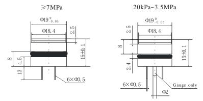
For option 0 or null, suggested installation dimension is  $\Phi 19^{+0.05}_{+0.02}$  mm.
