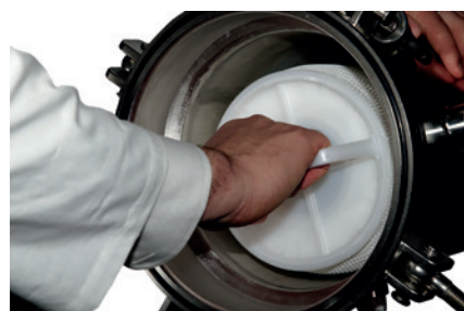
'Twist-to-lock' cartridge seating mechanism
