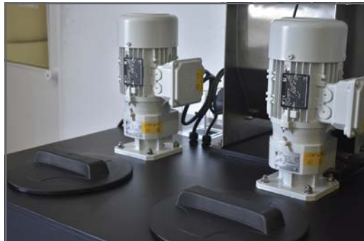
Round caps and special protective motor paint
