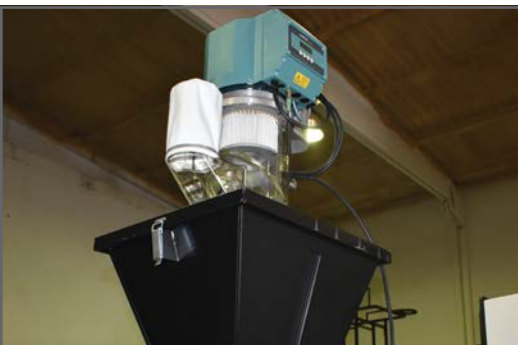
Automatic powder fill through vacuum hopper loader
