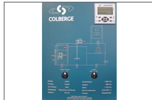
Synoptic panel w/ switches, signaling LEDs & graphical interface console
