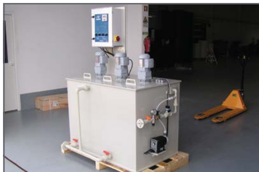
PP preparation tank
