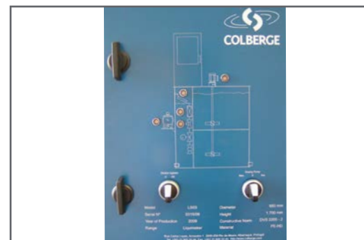
Control panel synoptic w/ switches & leds
