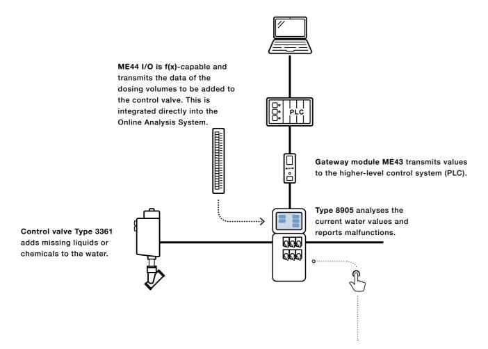
The configuration software "Bürkert Communicator" serves for parameterisation and diagnostic functions of the Online Analysis System. Cyclical values can easily be identified and displayed graphically. The f(x) graphical programming makes it possible to modify processes locally and individually without the need to intervene in the process control system.
