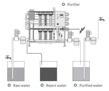
Membrane:Ultra-filtration10% Reject1500 l/h +Nano-filtration25% Reject1500 l/h +Reverse Osmosis30% Reject1500 l/h +
