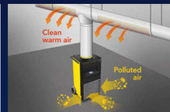
DualHeat blowing-out tower for an even distribution of warm air
